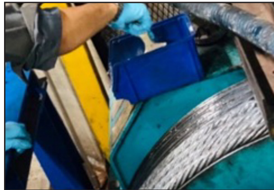
Chesterton 720 CCG with diluent applied with a brush on the wire rope.
